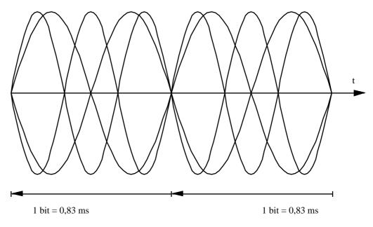
Fig. 4.6.3 Line diagram for the FFSK signal
