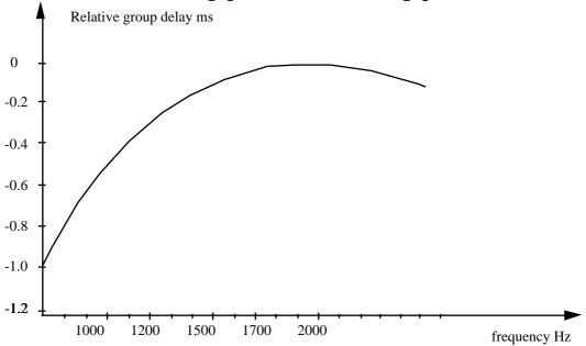
Fig. 4.6.5 Relative group delay of equalizer
