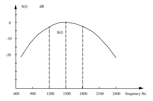
Fig. 4.6.4 Spectrum S(f) of the FFSK signal
